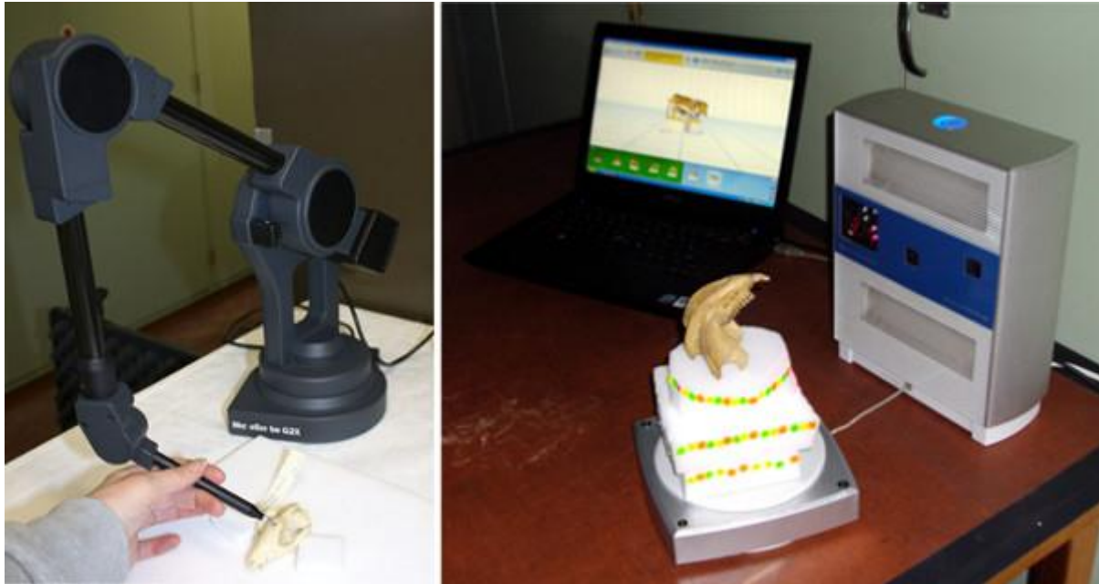
FIGURE 3 — A MICROSCRIBE (LEFT) AND LASER SCANNER (RIGHT).
