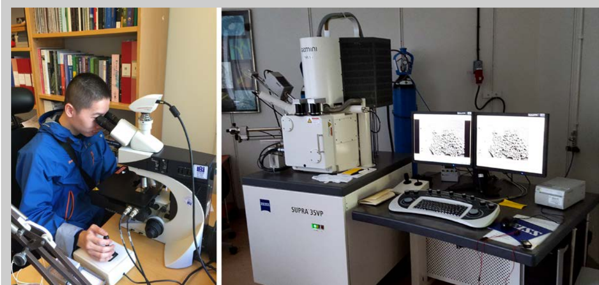
Figure 7 — Filtered residue containing the microfossils is mounted onto glass slides and studied by transmitted light microscope (left, credit: W. Taylor) and scanning electron microscope (right, credit: H. Agić.).
