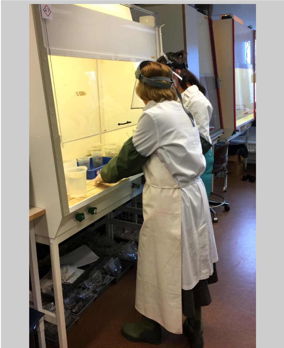
Figure 6 — Working with strong acids such as HF and HCl requires proper lab safety and protective equipment. A palynologist normally wears a collared lab coat, gloves (sometimes a double pair), rubber cuffs, apron, boots and eye protection. Credit: W. Taylor.
